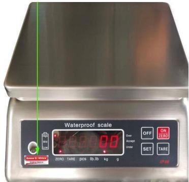
**DWP** is a high precision durable tabletop scale. it can give an accuracy of 0.5g on a 15kgs capacity. that being preferred by most of packaging industries. it is also a waterproof/dust proof/moisture proof weighing scale that can handle any wet environment and maintain the its high performance. it has a stainless-steel enclosure and rated to 1p69.comes with a rechargeable battery and internal power supply
